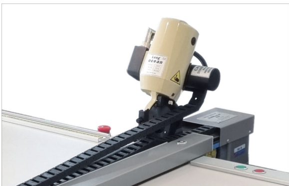
The Super Plus version equipped with an automatic cutter
