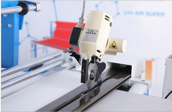
Super Plus version with DYDB-2B automatic end cutter
