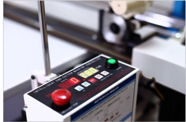
Control panel in Super and Super Plus versions features layer counter, setting the cutting length and the raising height of the cutting track.
